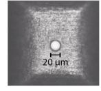
View down a laser-drilled square counerbore with a perfectly round hole in centre, with no stress cracking or carbonised debris.
